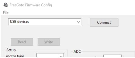
not connected the button besides the boardname shows "Connect" klicking on the button connects the program toe the Frego2-board. The button will show "DisConnect" to indicate that cliking ont the same button will disconnect the program from the freego2-board.
